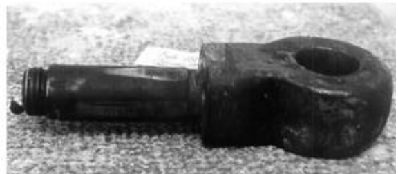
Figure 8. Detail of the broken buttonhole and bolt assembly.
