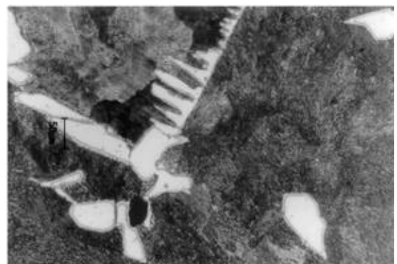
Figure 9. (X200) Microstructure of the wrought SAE 1045 bolt material. Widmastatten pearlite - ferrite ratio is 85/15.
