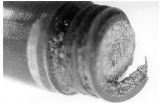
Figure 11. Fracture surface in the bolt . Note initiating defect within the first thread inside the fastener, and ligament torn by final plastic collapse.
