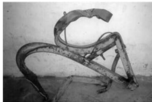
Figure 6. The lance was deformed by compression, bright scratches are found in its tip
