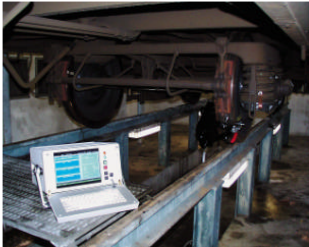
Figure 24. Base unit of the portable UER-T set-up for the automated evaluation of stress states of wheels.
