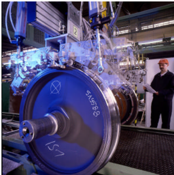
Figure 4. Transducer system carrier being positioned to the wheel.
